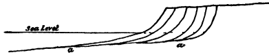
FIG. 43.—To show the advance of the sea, making a plain of marine denudation from a to a' .
